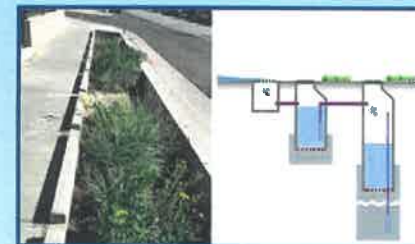
Rainwater Catchment System
