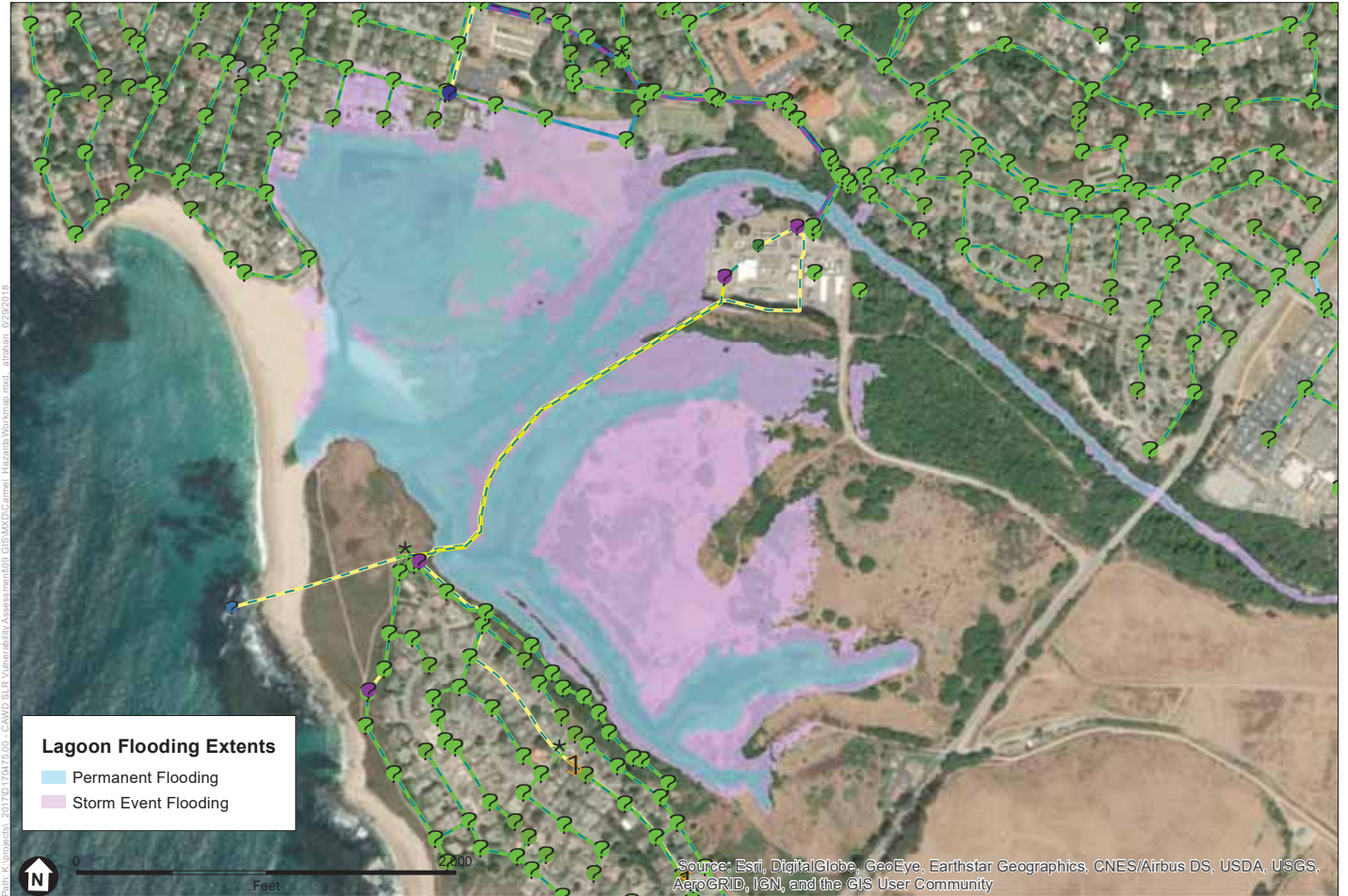
CAWD SLR Vulnerability Assessment . D170475.00 Figure 10 CAWD Asset Exposure Lagoon Flooding under Existing Conditions
