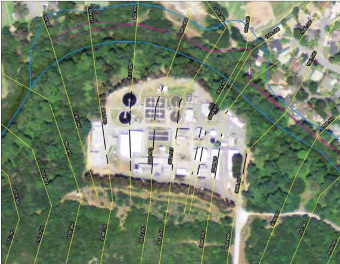
Figure 2: Treatment Plant Obstructions (shown in Black)
