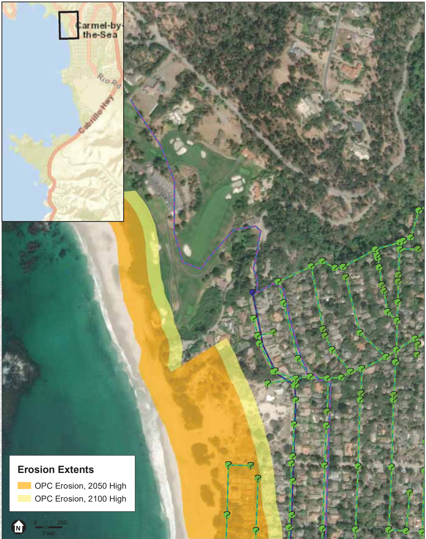
Figure 13 CAWD Asset Exposure Shore Erosion
