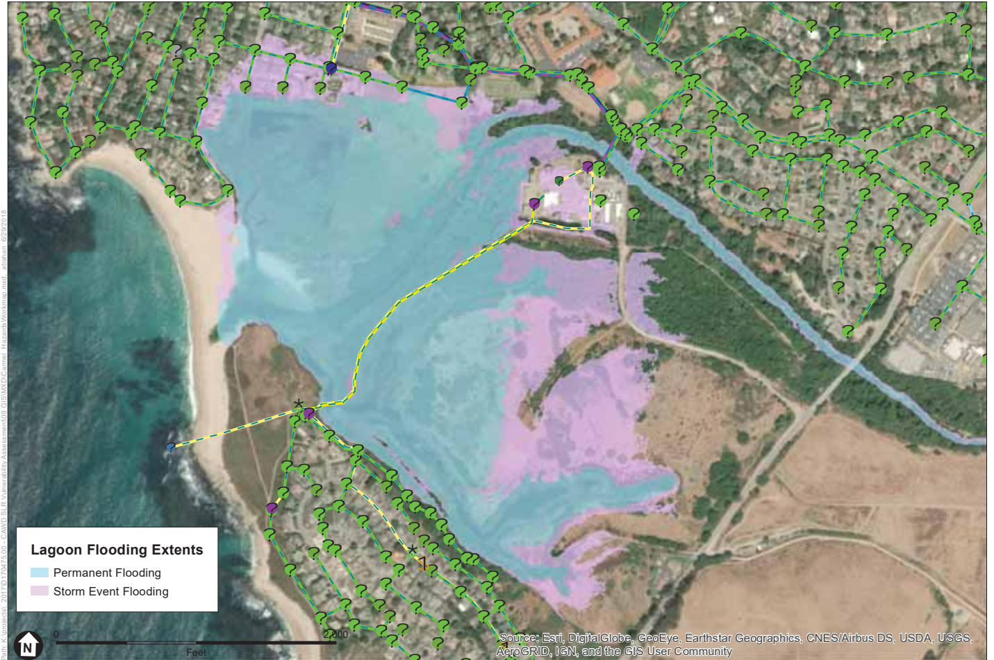
Figure 11 CAWD Asset Exposure Lagoon Flooding at 2050
