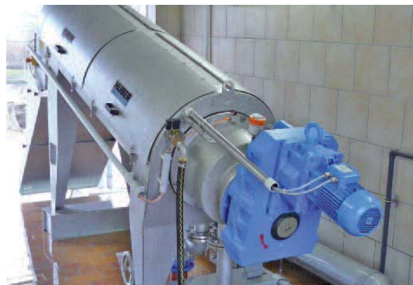
Screw press for 24/7 unattended operation
