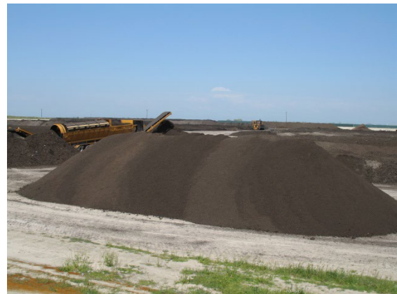
Central Valley Compost Facility. At our Central Valley Compost facility, Synagro utilizes a mobile chip and grind operation for inbound feedstock size reduction.
