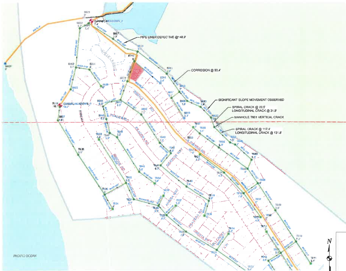
0 225 APPROXIMATE SCALE IN FEET Kennedy/Jenks Consultants CARMEL AREA WASTEWATER DISTRICT CARMEL MEADOWS GRAVITY SEWER SUMMARY OF 6-INCH GRAVITY SEWER CONDITION ASSESSMENT JULY 2013 (FWY) 1399011\FIG-01 FIGURE 1
