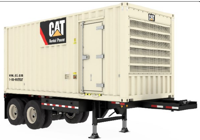
Photo: Example Trailer Standby Generator
