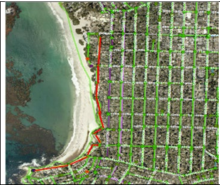
Photo: Pipe Bursting Limits on Scenic
