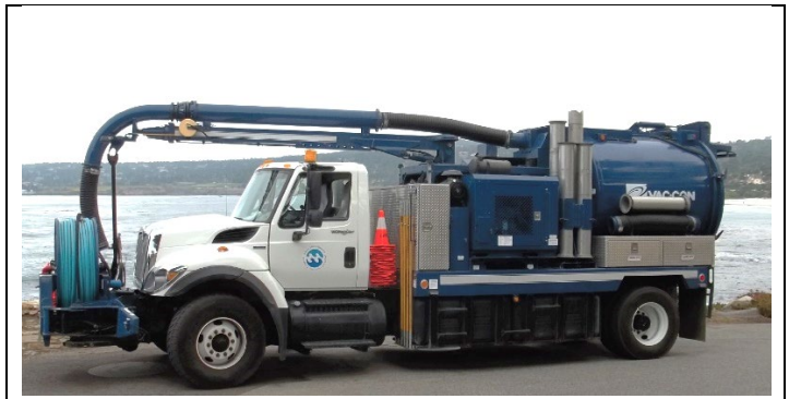
Photo: CAWD Vactor Truck
