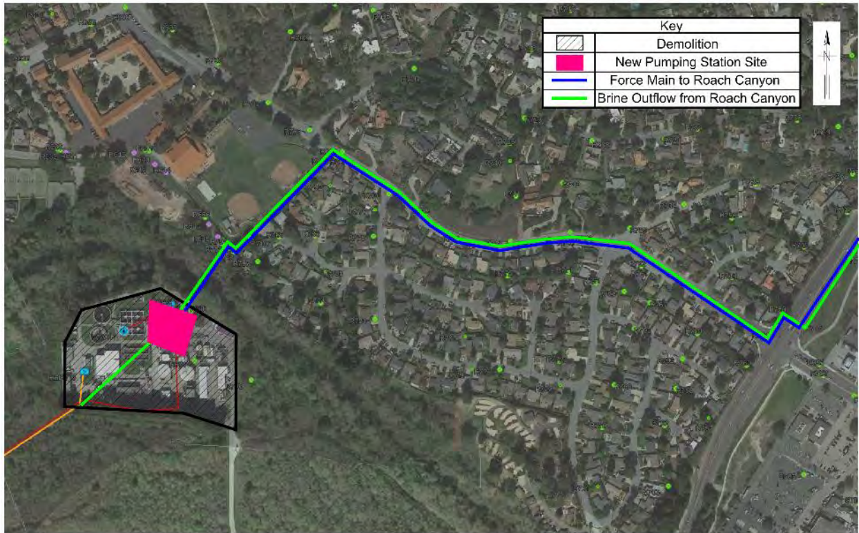
Figure 3-5: Conceptual Routing for Alternative 1
