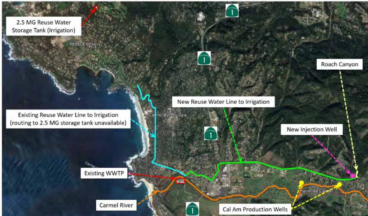
Figure 3-15: Conceptual Connection Piping from the WRRF to the Existing Reuse Water Line
