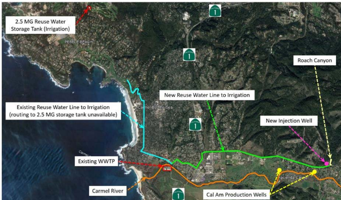
Figure 4 – Centralized WRRF Reclaimed Water Conveyance
