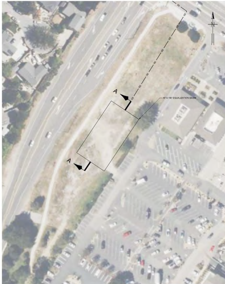
Figure 3-13: Conceptual Site Layout of EQ Basin at Hatton Canyon Park
