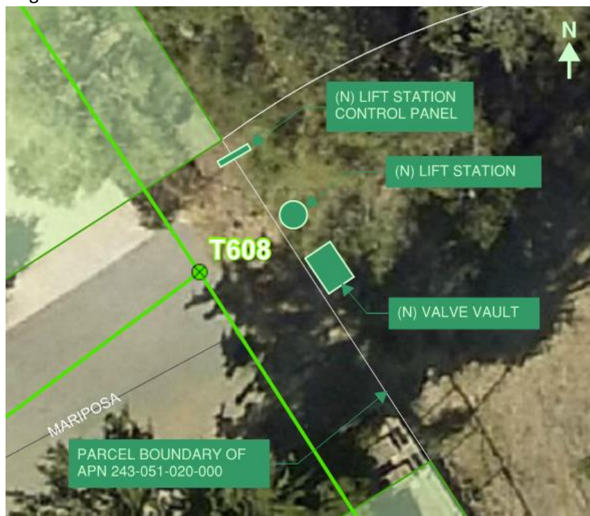
Figure 8. New Lift Station Location and Layout Alternative 1
