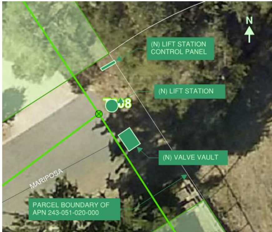
Figure 9. New Lift Station Location and Layout Alternative 2
