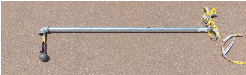
Image 4 – Diffuser sounding device
