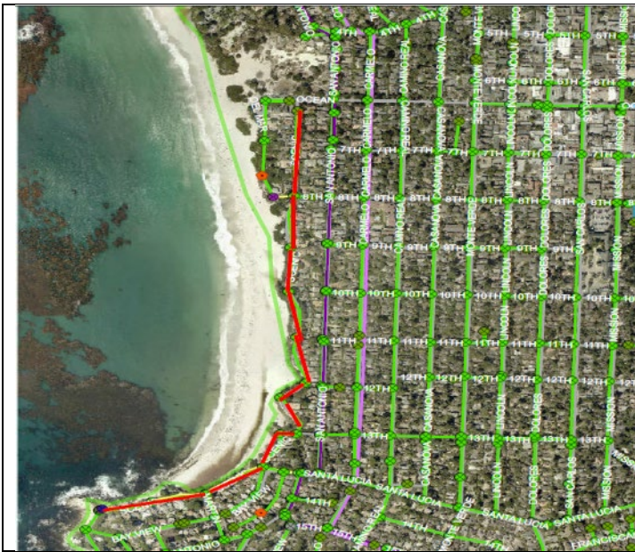
Photo: Pipe Bursting Limits on Scenic
